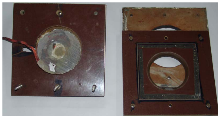
Figure 2. Assembly photograph of the actuator coil and forming fixture
