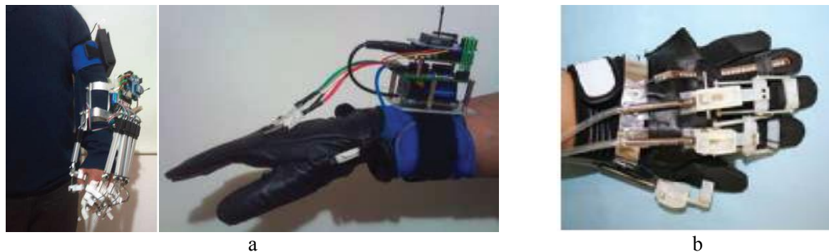
Figure 2. Exoskeletons: a) exoskeleton control glove [4]; b) PAFEx [5].
