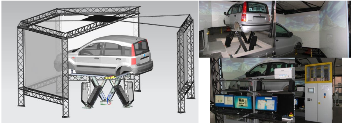
Figure 1. Virtual model and the real system of the simulator for car driving learning.
