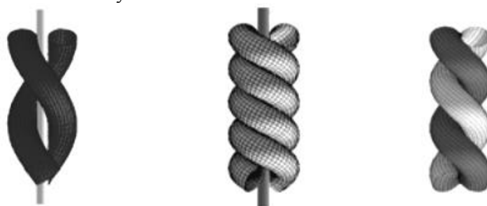
a. Metal-wrapped yarn b. Metal-filled yarn c. Metal yarn
