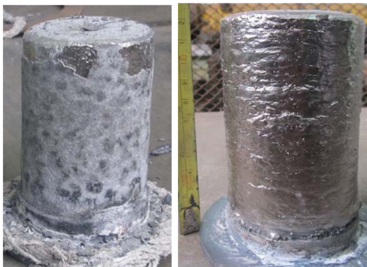
Figure 4: Obtained ingots after electroslag remelting before (left) and after (right) slag skin removal
