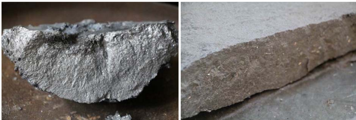
Figure 2: Cross Section of small scale (left) and large scale (right) ATR products
