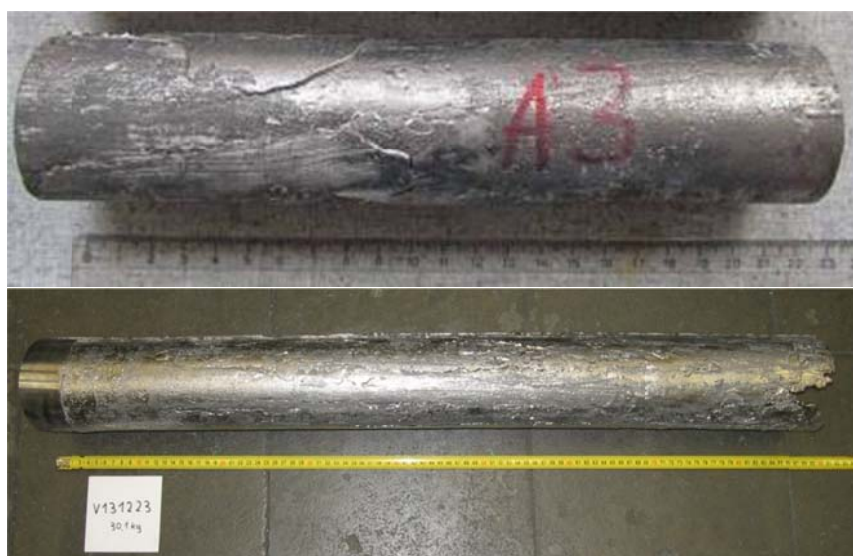
Figure 3: Obtained Electrode after pilot scale VIM, top: lab scale, bottom: pilot scale
