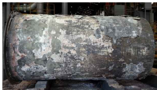
Figure 14. Appearance of 120ton-class 9CrMoCoB Steel of ESR ingot
