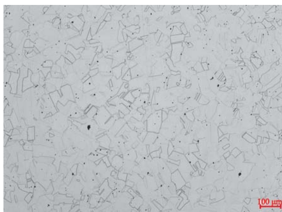
Figure 11. The microstructure of HNS-A after solid solution treatment.
