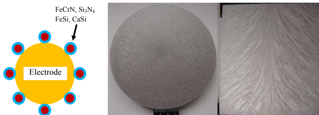
Figure 12. Composite electrode and Macrostructure of P2000 ingot made by PESR.
