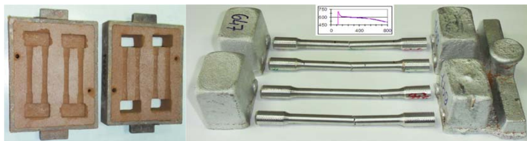
Figure 1. (a) Sand mould for tensile strength and elongation measurements ; (b) Machined specimens after UTS tests with risers and gating system.
