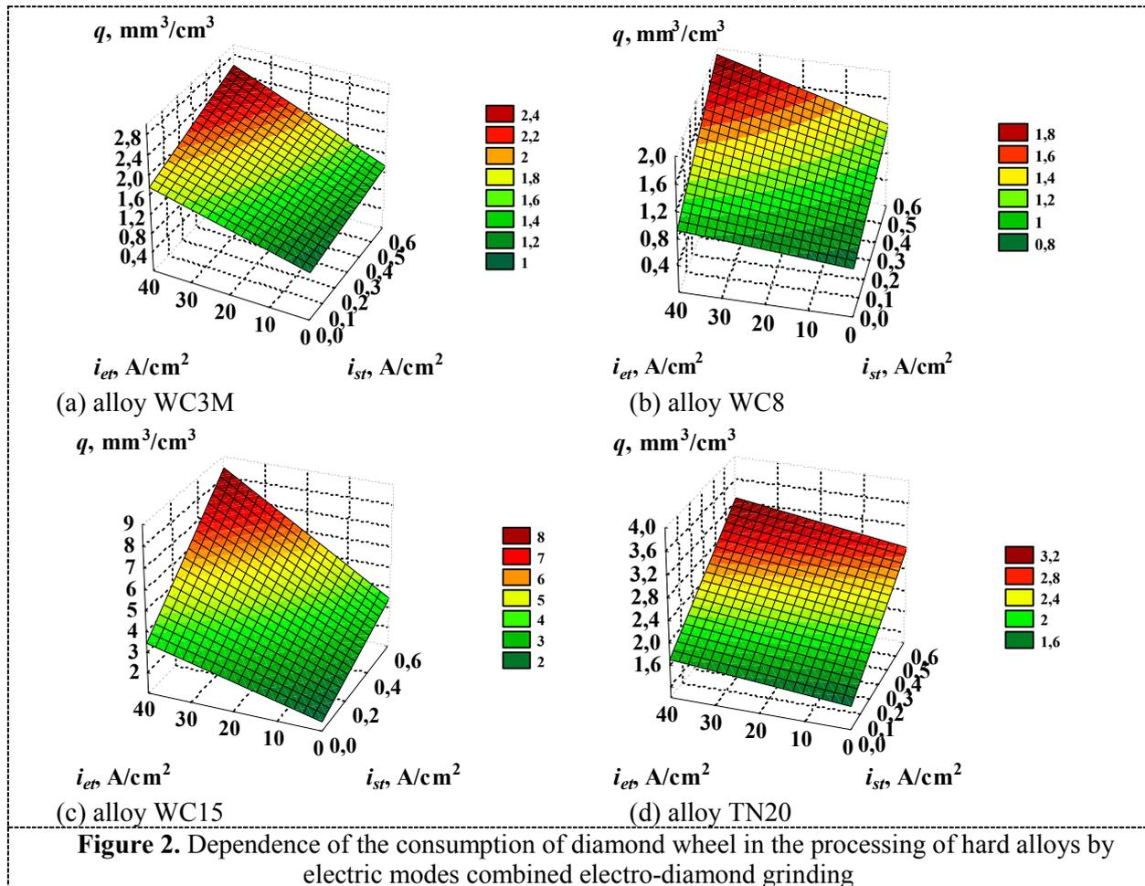
Dependence the consumption of diamond wheel  $q$  [ $\text{mm}^3/\text{cm}^3$ ] from electrical modes  $i_{st}$  [ $\text{A}/\text{cm}^2$ ] и  $i_{et}$  [ $\text{A}/\text{cm}^2$ ] for alloy WC3M has the form:
