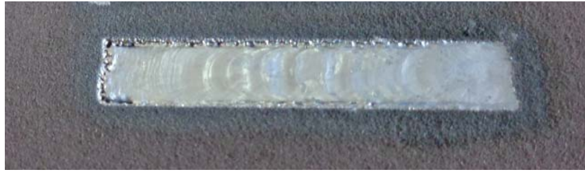
Figure 2. Sintering the rectangular samples of copper powder.
