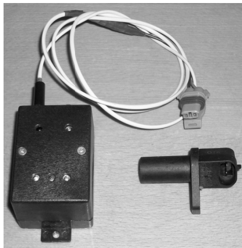
Picture 3. – Indicator with the transducer and the sensor (left)
