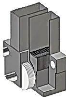
Figure 7. The multi-nozzle dispensing feeder with dispensing roller consisted of a set of thin discs (about 1mm), each of which is equipped with individually controlled drive.
