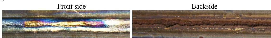
Figure 4 – The appearance of joint weld performed at LTW with welding velocity V_{\text{weld}} = 0.72 m/min
