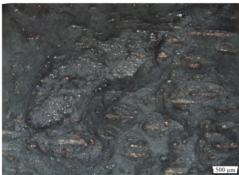
Figure 2. Type of fracture of the sample with lower plastic properties
