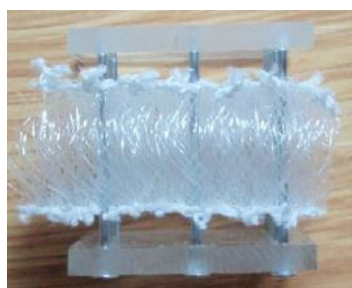
Figure 7. Apparatus for micro CT-scanner SkyScan 1174
