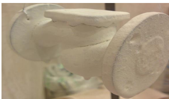
Figure 6. Model with the deposited refractory coating after 12 hours
