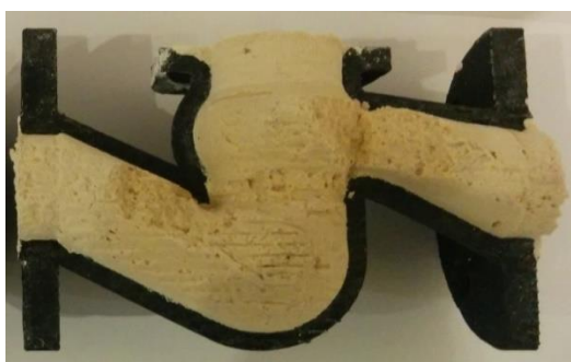
Figure 5. Rammed core in the model
