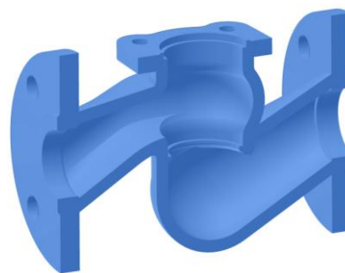
Figure 2. Design of cast valve body for 3D printing
