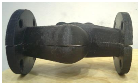
Figure 4. Model after machining the parting plane
