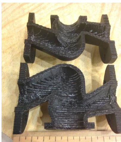
Figure 3. Inner surface of ABS-model after removing the pattern-supporting layer
