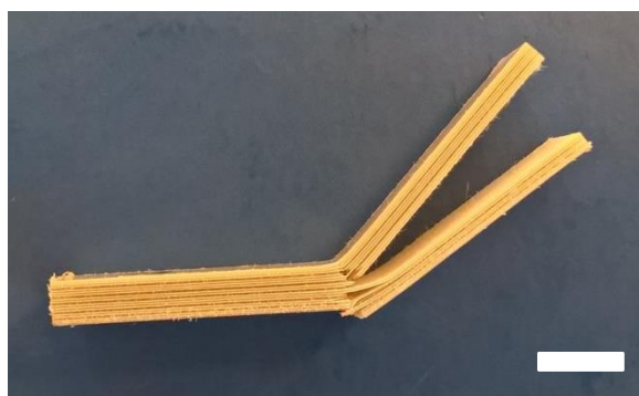
Figure 7. Exemplary fractured test specimen from ILSS impact testing exhibiting laminar failure (scale bar represent 5 mm)
