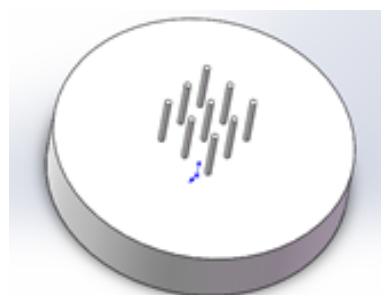
Figure 1. The micro-needle array model obtained through the SolidWorks software
