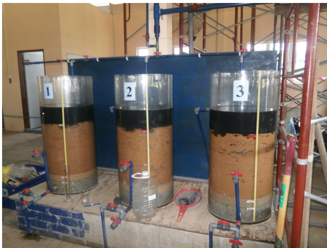
Figure 2. A soil column experiment in treating stormwater pollutants.
