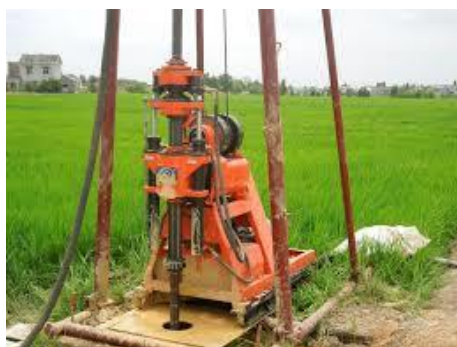
(f) Standard Penetration Test (SPT)
