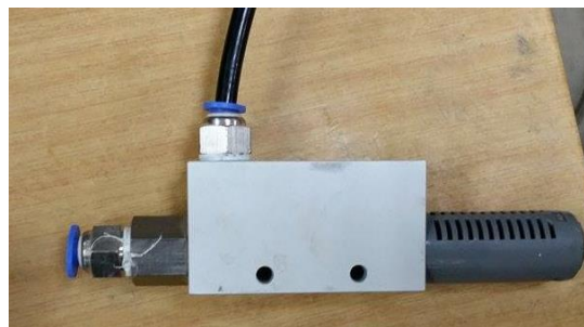
Figure 3. Convum installed at cell pressure and back pressure inlets.
