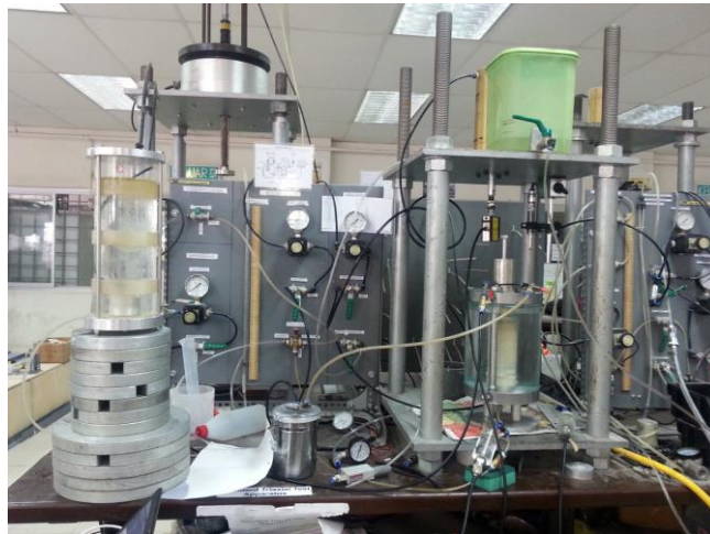
Figure 2. Photograph of the actual Consolidated Undrained Triaxial setup.
