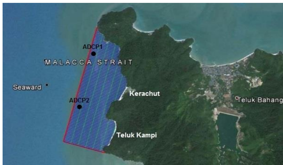
Figure 3. Transect line for bathymetry survey.
