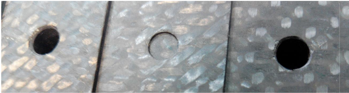
Figure 4. Flat-bottom holes on the reference sample.
