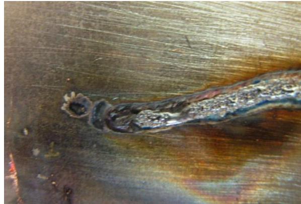
Figure 2. Traces of melting on the surface of processed part after the low-temperature plasma treatment.
