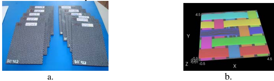
Figure 1. Studied samples: a) composite plates; b) 5 Harness satin fabric layout.
