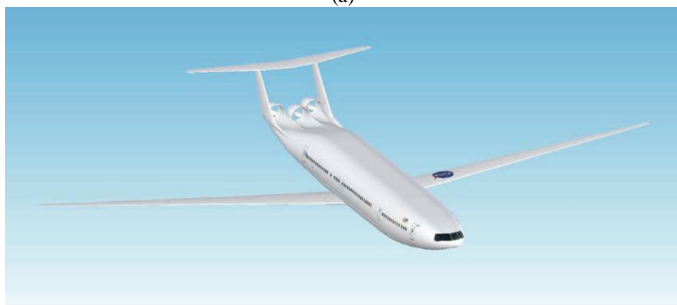
Figure 9. New concept of aircraft design for open-rotor and turbofan high bypass ratio engine: a) Lockheed Martin's box-wing concept [18], and b) MIT's double bubble concept [19].
