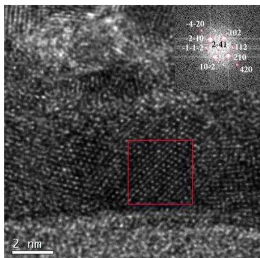
**Figure 2.** Bright-field HRTEM image of a cross section of the irradiated NbN film at a dose of  $\sim 1$  d.p.a. for nitrogen, diffraction pattern (inset).
