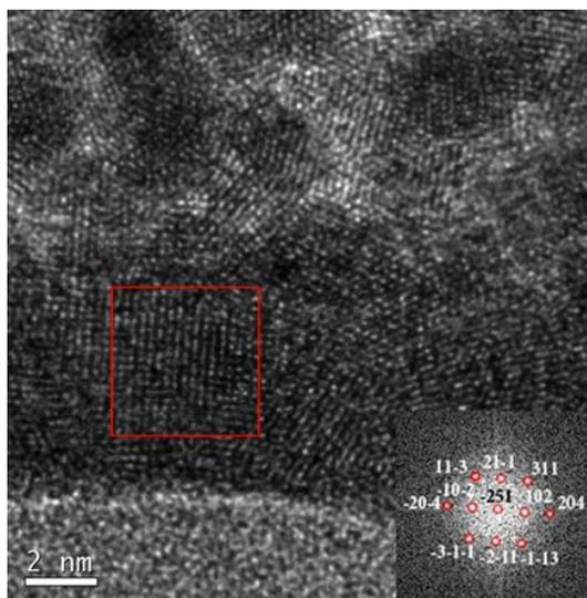
**Figure 3.** Bright-field HRTEM image of a cross section of the irradiated NbN film after composite irradiation to a dose of  $\sim (1.5-2)$  d.p.a. for nitrogen, diffraction pattern (inset).
