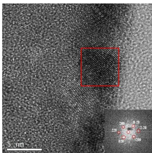
**Figure 1.** Bright-field HRTEM image of the cross section of the film NbN, synthesized on a substrate of SiO<sub>2</sub>, diffraction (inset).
