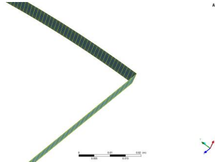
Figure 12. The mesh detail of the internal clearance flow area.
