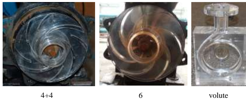
Figure 2. Impellers and volute of model pump
