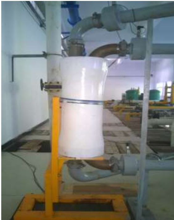
Figure 4-1. The figure shows that the energy recovery device is in field application. The location of the field application is in Changtu desalination factory in Daishan County in Zhoushan City. The amount of processing of this factory achieves 5000\text{m}^3/\text{d} [8]. The field application was operated by plunging the energy recovery device into technological process of the desalination factory.
