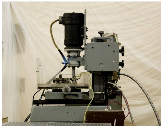
Figure 1. The scheme and appearance of an experimental facility for electro-diamond grinding. 1 – diamond disk on a metal alloy; 2 – test specimen; 3 – strut for fixing the test specimen; 4 – electrochemical cell; 5 – ball bearing ways; 6 – pedestal base; 7 – feed motor; 8 – primary motor; 9 – carriage; 10 – spindle; 11 – contact-wiper facility; 12 – DC source–VSA 5; 13 – voltage source; 14 – joint box; 15 – cleat; 16 – lead screw; 17 – fixing screw; 18 – isolating joint box; 19 – textolite washer; 20 – cell limit stop.
