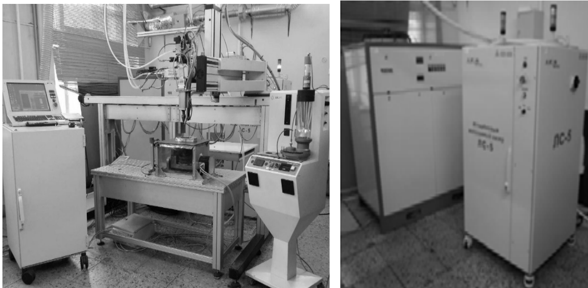
Figure 1. Laboratory bench for studies of the process high-speed direct laser deposition.
