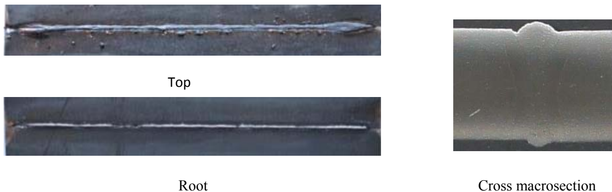
Figure 4 - The appearance of weld (Sv-10H19N11M4F)
