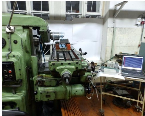
Figure 2. A system for experimental studies of plastic insulators cutting
