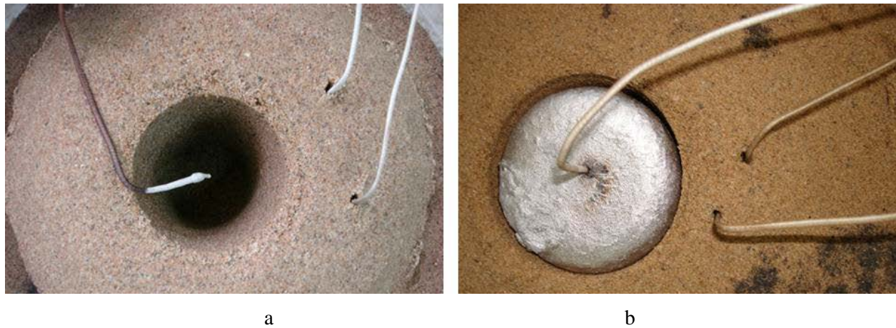
Figure 2. The casting mold with defined thermocouples (a) and the experimental casting (b) for determination of the heat storage capacity of the mold.
