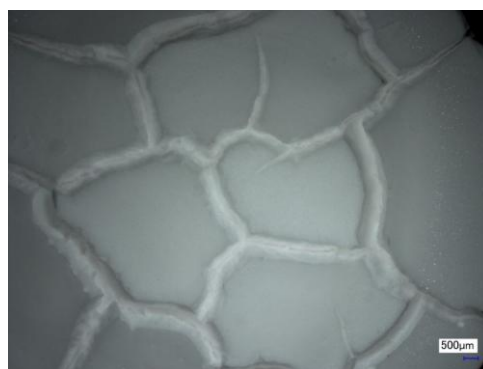
Figure 3. Surface defects – cracks – on optical microscope
