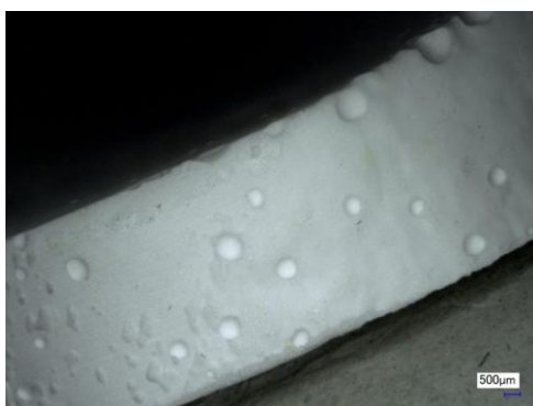
Figure 2. Surface defects – bubbles – on optical microscope
