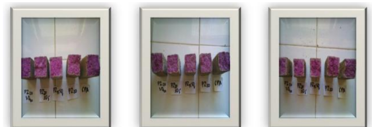
Figure 3. Phenolphthalein indicator staining specimens attacked by HCl, H 2 SO 4 and (NH 4 NO 3 + HNO 3 )
