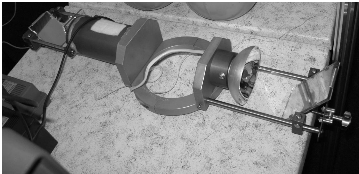
Figure 2. The appearance of the system of video observation for electron beam welding process
