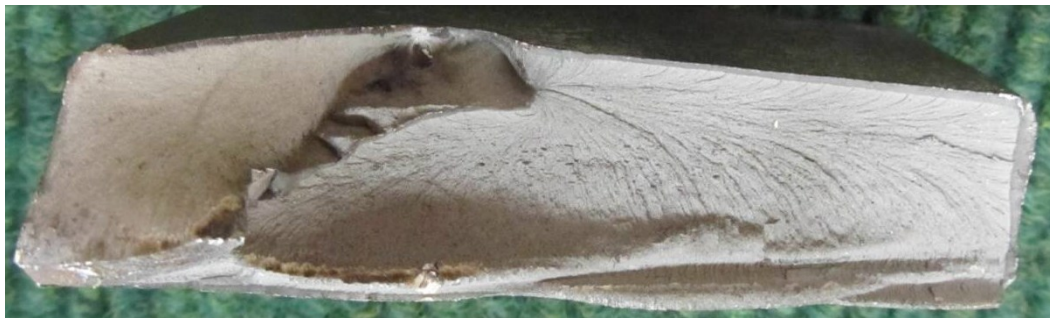
Fig. 1. Leaf spring bar section with inclusion around 0.4 mm under surface at distance 0.8 mm
