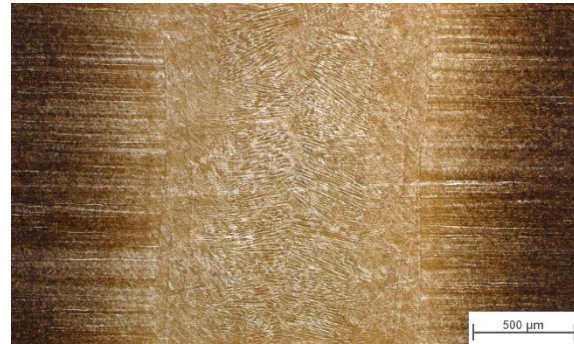
Figure 10. 20mm weld, Ra6.3, no pores visible
