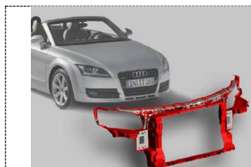
Figure 1. Audi TT front end carrier [2]
