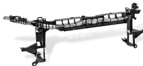
Figure 2. Mercedes B class front end carrier [3]
