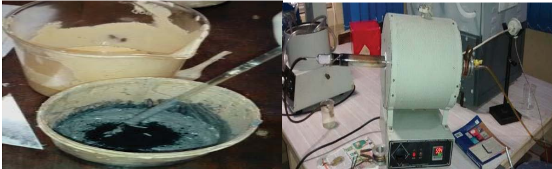
Fig. 1:- Abrasive laden Media (carrier+Al 2 O 3 +CNT) Fig.2. Thermal CVD Setup Fe-filled CNTs.
