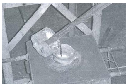
Figure 2: Pouring of Al-SiC melt into mold.
