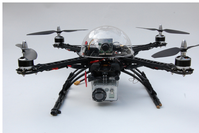
Figure 9. Design of UAV with night vision camera
