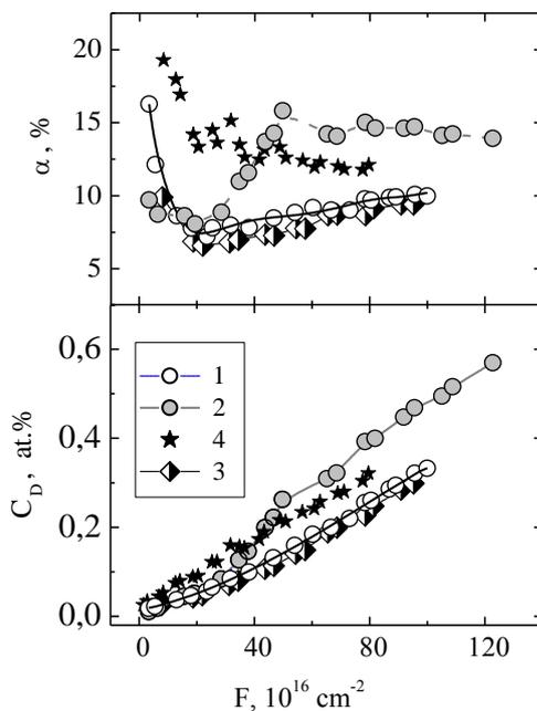
Figure 1. The effect of radiation dose  $F$  on  $C_{\text{D}}$  and  $\alpha$  for Kh15N16M3T1 steel samples.
