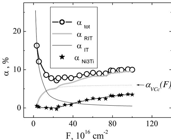
Figure 2. The scheme of decomposition of total deuterium capture  $\alpha$  into trapping capture in hardened sample of steel Kh15N16M3T1
