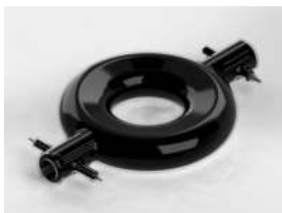
Figure 1. Sealed vacuum acceleration chamber of 6 MeV betatron.
