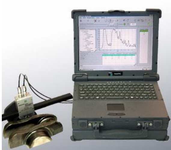
Figure 3. Ultrasonic testing instrument for testing the case depth, P3121, Case Depth Tester.
