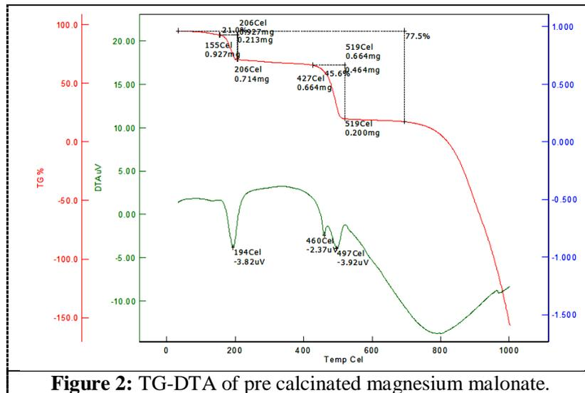
**Figure 2:** TG-DTA of pre calcinated magnesium malonate.
