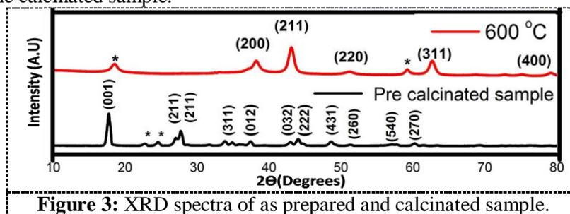
**Figure 3:** XRD spectra of as prepared and calcinated sample.
