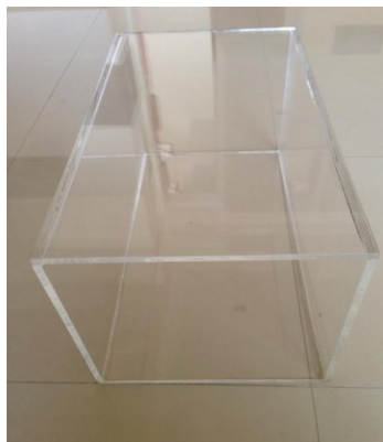
Figure 3. Photograph of actual test section made from plexiglass.
