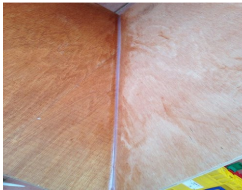
Figure 4. Joint filled with silicone glue (top view).
