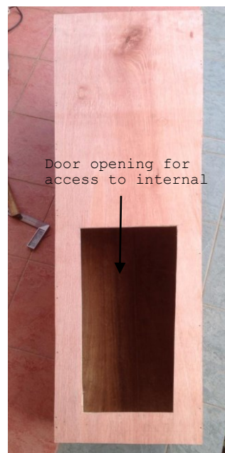
Figure 7. Trapezium shape diffuser made of plywood.
