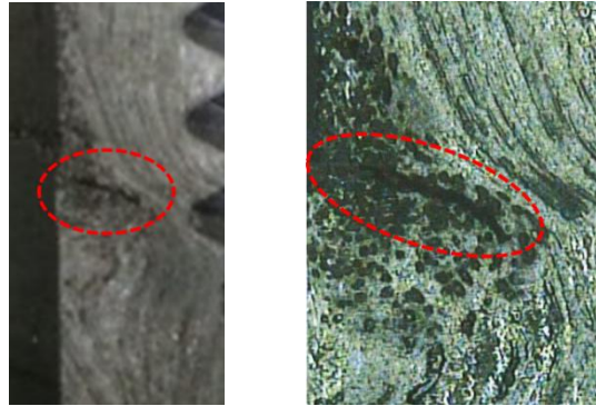
Figure 1. Internal defect of 1 mm size caused on the oil filter bolts
