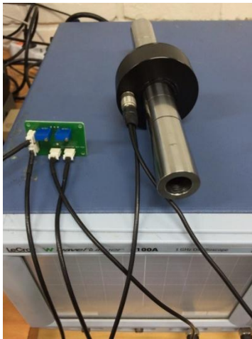
Figure 13. Finally designed differential bobbin probe.
